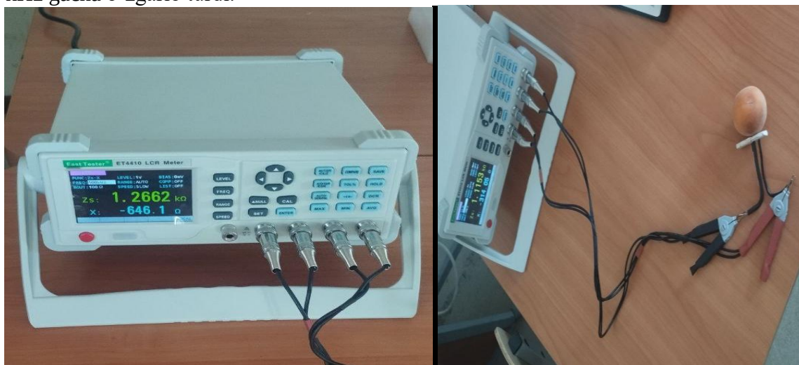
2-rasm. mevalarning impedansini o’lchash jarayoni
