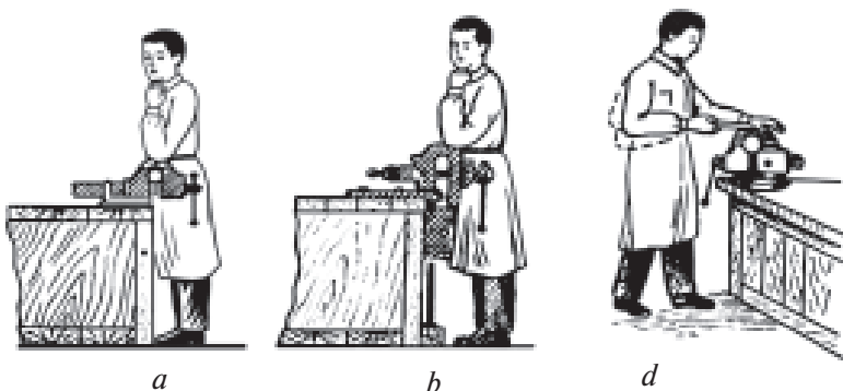
5-rasm. Ishchining bo‘yiga qarab parallel va stul tiskilarning verstakka o‘rnatilishini tekshirish
