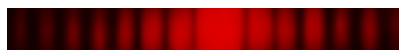
w / Single-slit diffraction of red light. Note the double width of the central maximum.
