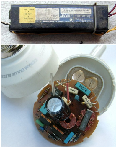
n / Ballasts for fluorescent lights. Top: a big, heavy inductor used as a ballast in an old-fashioned fluorescent bulb. Bottom: a small solid-state ballast, built into the base of a modern compact fluorescent bulb.
