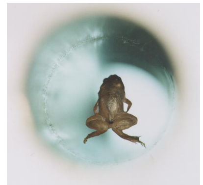
h / A frog is levitated diamagnetically by the nonuniform field inside a powerful magnet. Evidently frog has \mu < \mu_0 .
