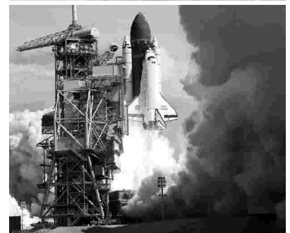
r / The wheel spinning in the air has K_{cm} = 0 . The space shuttle has all its kinetic energy in the form of center of mass motion, K = K_{cm} . The rolling ball has some, but not all, of its energy in the form of center of mass motion, K_{cm} < K . (Space Shuttle photo by NASA)
